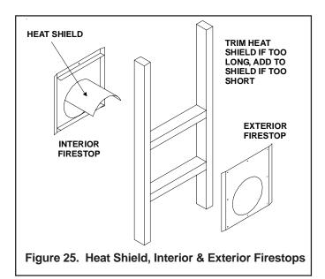
**For Vertical Runs -** One ceiling firestop is **REQUIRED** at the hole in each ceiling through which the vent passes.
